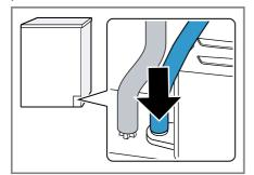
4. Insert the water drain hose into the hose guide.
