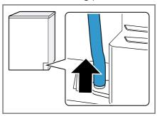
The condensation hose is connected to the connecting piece at the factory.
